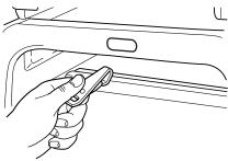
4. Rotate the tether hook, and clip the tether strap to the seat frame.
